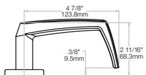
1. Complies with codes requiring lever to return to within 1/2" (13mm) of door face.
