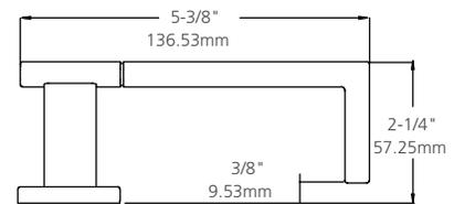
1. Complies with codes requiring lever to return to within 1/2" (13mm) of door face.
